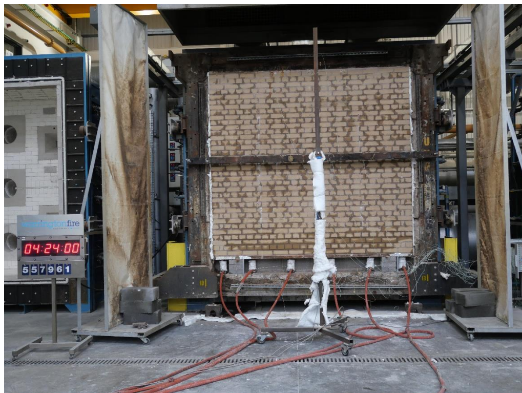
The unexposed face of the wall assembly at the termination of the test
